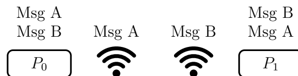
Figure 3. Two senders transmits messages A and B at the same time, because of physical proximity process zero will receive the messages in the order A then B , while process one will receive them in the order B then A . This is still a correct reliable broadcast.
