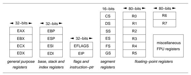
Figure 3: Registers in IA32 processors
