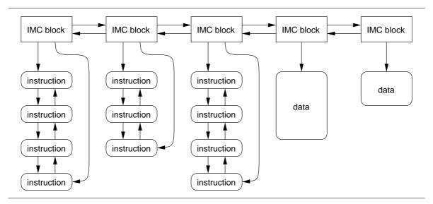
Figure 5: Internal program representation in tranx86
