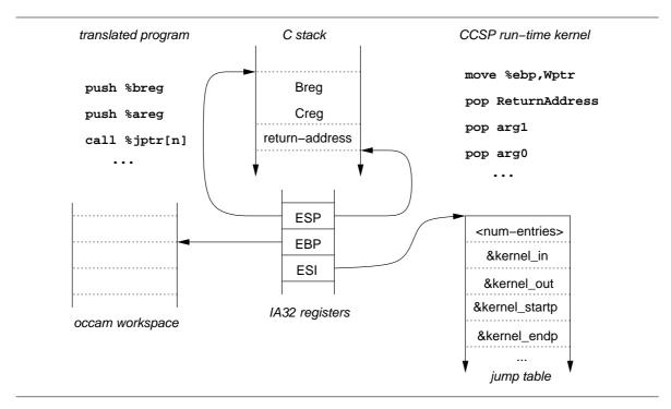
Figure 6: Original run-time kernel calling sequence
