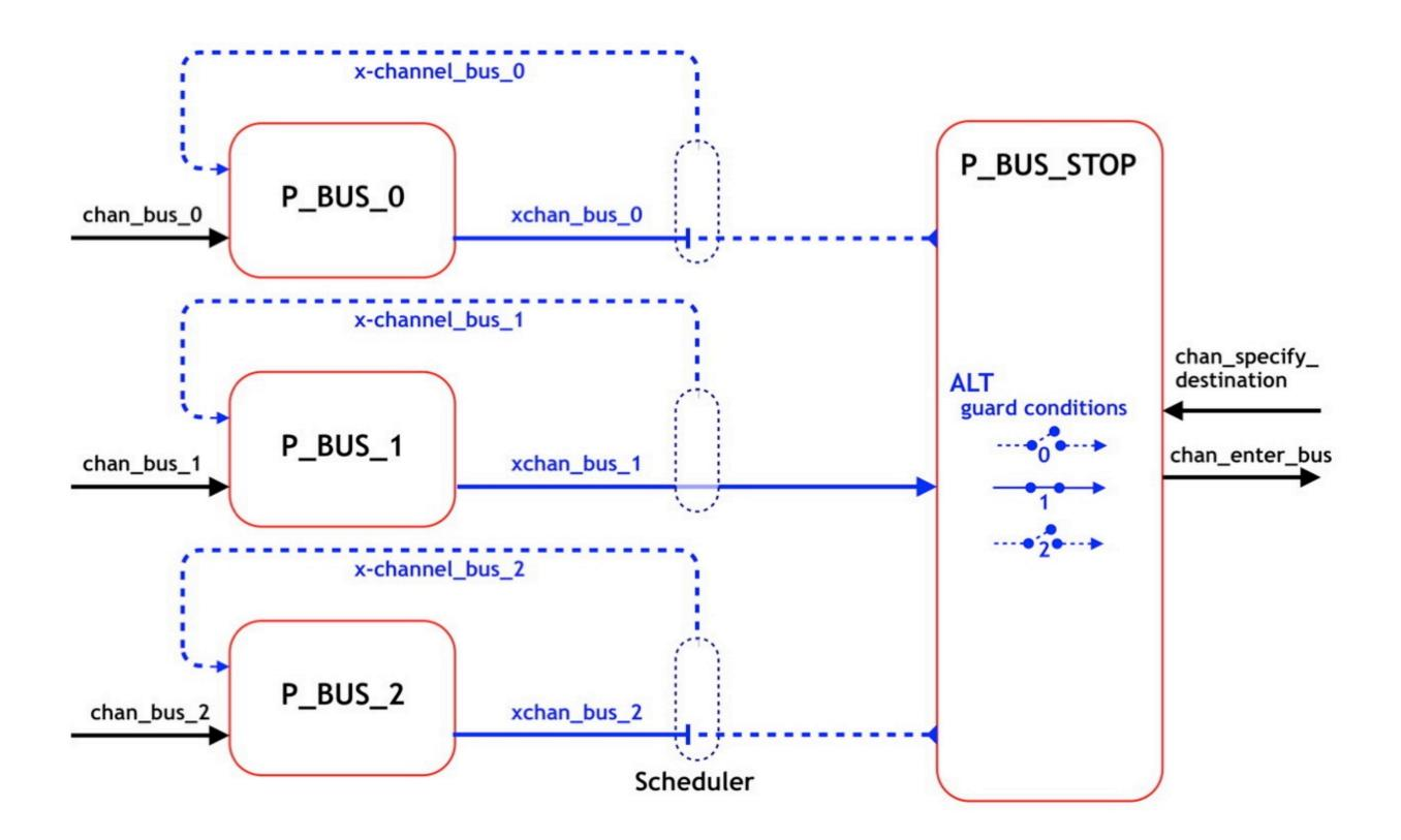
Figure 2. XCHAN (array of 3) and feathering, with only bus #1 as possible to ride
